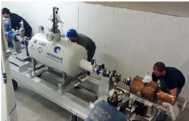
Figure 2. A compact superconducting accelerator used for radioisotope production
